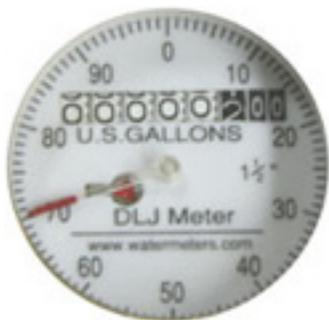
**Pulse Output** The DLJ line is available with a dry contact reed switch pulse output. This requires external DC power, 4 watts, 30VDC maximum. Contact closure is 1 pulse per 10 gallons.
